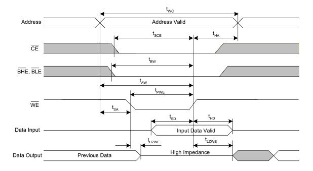
21.  $\overline{\text{CE}}$  or  $\overline{\text{WE}}$  must be  $\geq V_{\text{IH}}$  during address transitions.
